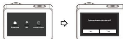
2. Follow the instructions and press and hold both buttons at the same time. To connect the remote control to the camera.
